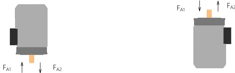
Standard design with deep groove ball bearings
